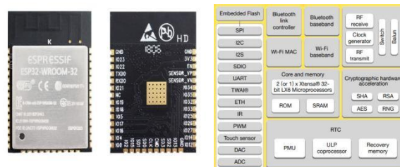
Fig b. This figure represents the microcontroller and the internal structure of ESP32.
