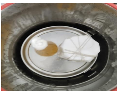
Fig 3: Autoclaving the Petri plates & nutrient agar
