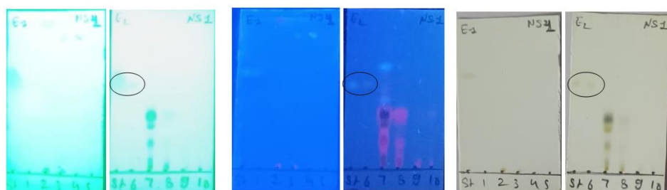
Figure 4 TLC estimation by UV lamp for NS fractions after column chromatography with Std. terpenoid (Carvacrol) a) Short-UV (254 nm), b) Long-UV (365 nm), c) visible light (Std. = Standard, NS= Nigella sativa )
