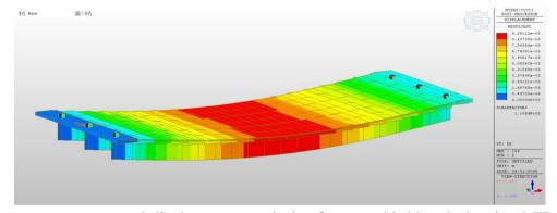
The image represents a structural displacement analysis of a curved bridge deck using MIDAS software. The colour gradient gives the displacement levels under dead load (DL), with blue is the minimal displacement and red represents the maximum displacement at the central .The support locations are
