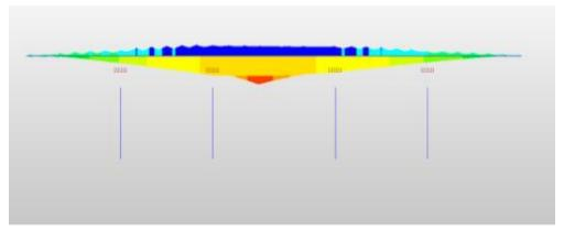
The image represents a structural stress distribution analysis of a bridge, likely depicting shear force or stress contours obtained from MIDAS software. The colour variation gives the info of intensity of bending moment. This analysis is important for ensuring high-stress zones, ensuring that reinforcement is provided in critical areas to increase the bridge's durability and structural integrity.
