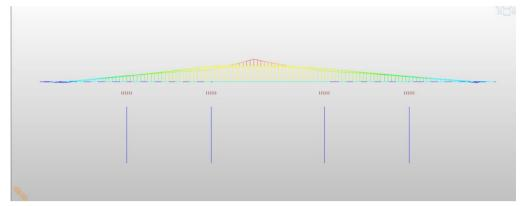
The image is a structural analysis result from MIDAS Civil, displaying the bending moment distribution of a multi-span bridge. The colour variation mainly shous about the intensity of deflections.Red region experiences maximum and blue region experiences minimum.
