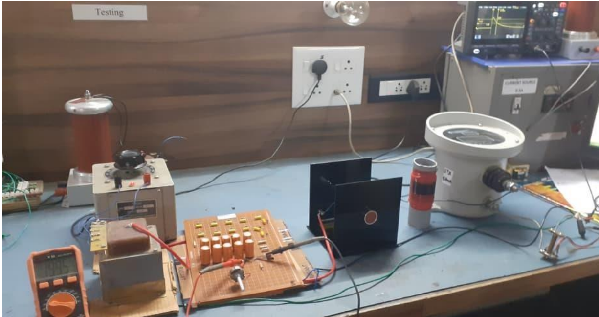
Figure 6.2: Surge Counter Testing kit
