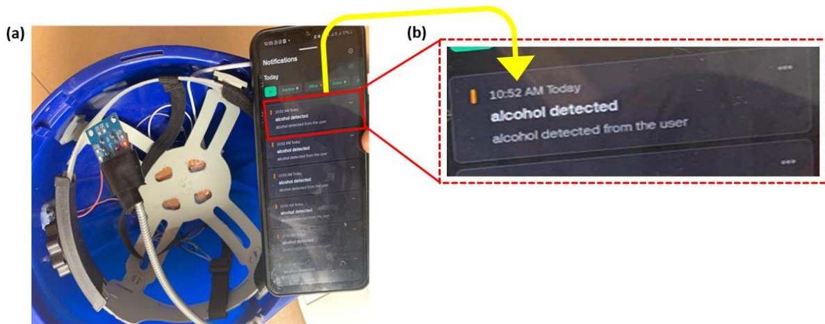
Figure 9: (a) Smart helmet system design setup (b) magnified message of alcohol detection by user to the supervisor
