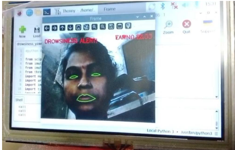
Figure 4: Drowsiness detection screen of raspberry pi 4B
