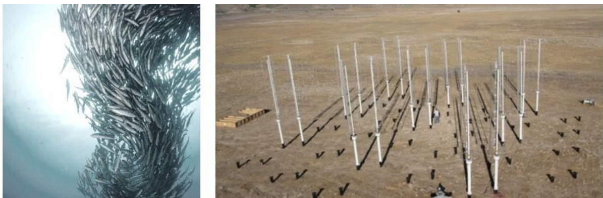
Figure 26. (a) Shoaling fish swim in formations that optimize the use of eddy currents (b) Scientists have applied the principles in vertical wind turbines for a demonstrated substantial increase in energy generation (Source: Pawlyn, 2019)
