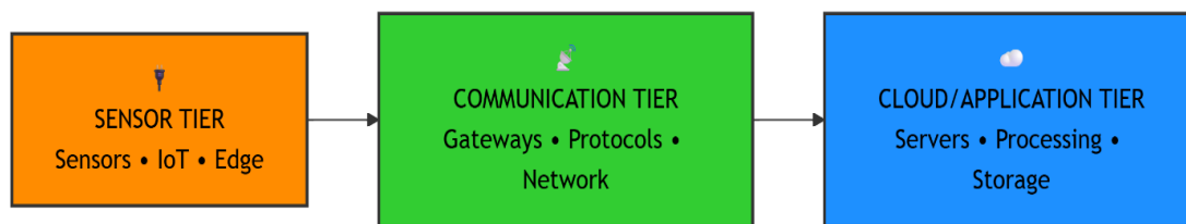
Figure 1: Architecture Tiers of an IoT System
