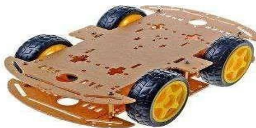
Fig. 1. Four-Wheel Robot Chassis Used for the Firefighting Robot
