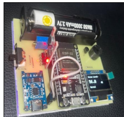
Figure 5: Prototype of the IoT Enabled Real-Time Noise Surveillance Monitoring Device showing the ESP32, sound sensor, LCD display, buzzer, and power supply on the PCB
