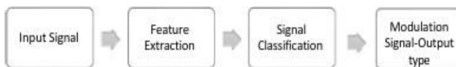
Figure 3.1: Proposed system block diagram showing signal flow from input acquisition to classification.
