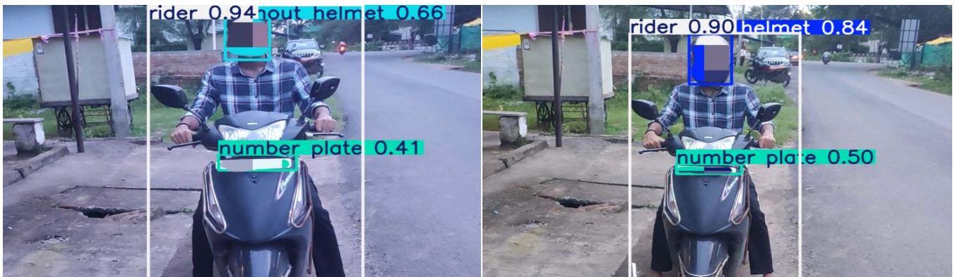
Fig 3. Output Example of Multi-class Object Detection
