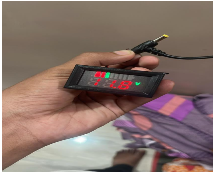
Fig 3. Battery voltage display during charging
