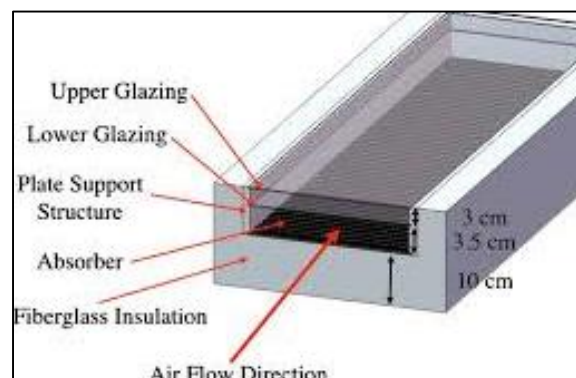
Fig: -3.2 Components of Solar Air Heater
