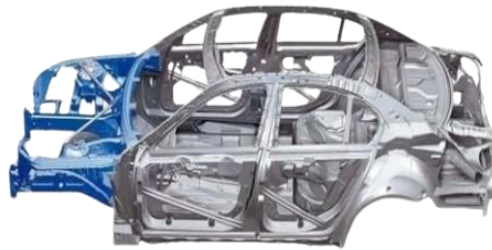
Fig. 3.2 Monocoque Chassis Architecture Image Source: slideshare
