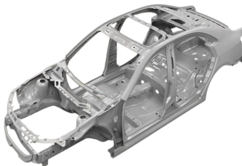
Fig. 2.3 Advanced High Strength Steels (AHSS) Manufactured Vehicle Chassis Image Source: Nationalmaterial.com
