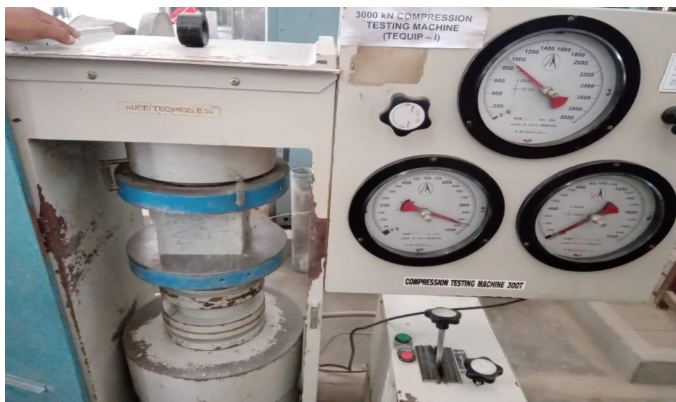
Figure 4.6 Compressive strength on cube
