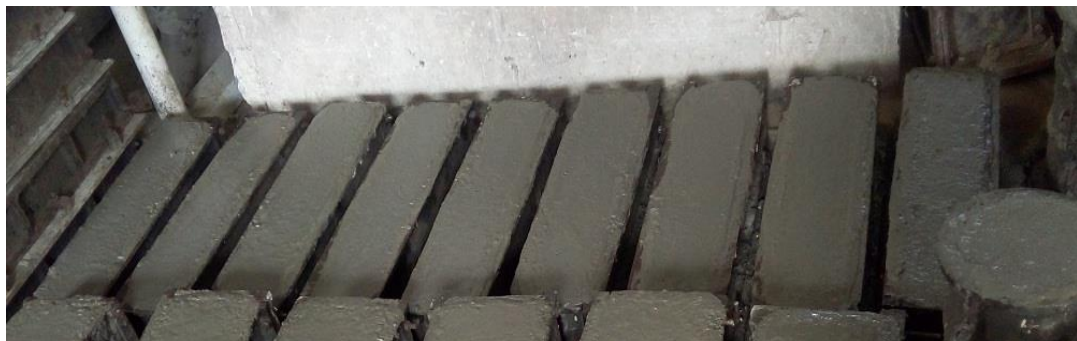
Figure 4.5 Casting of prisms
