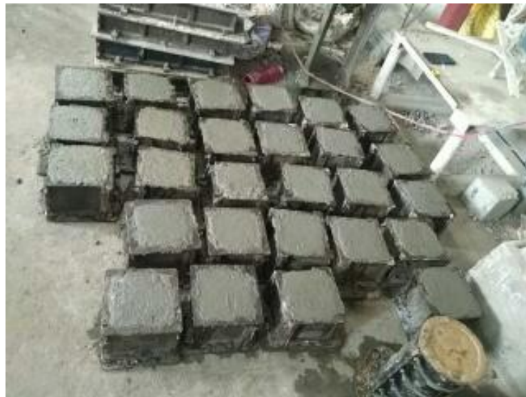
Figure 4.3 Casting of cubes
