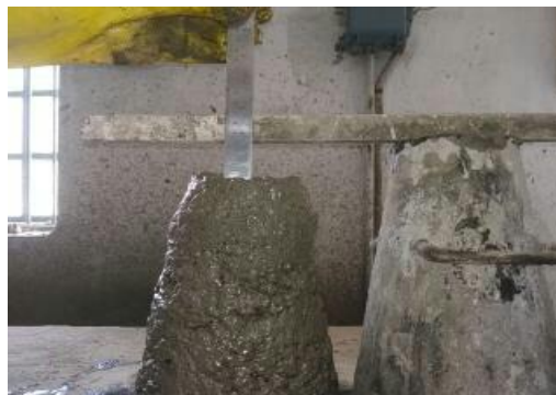
Figure 4.1 Slump cone test
