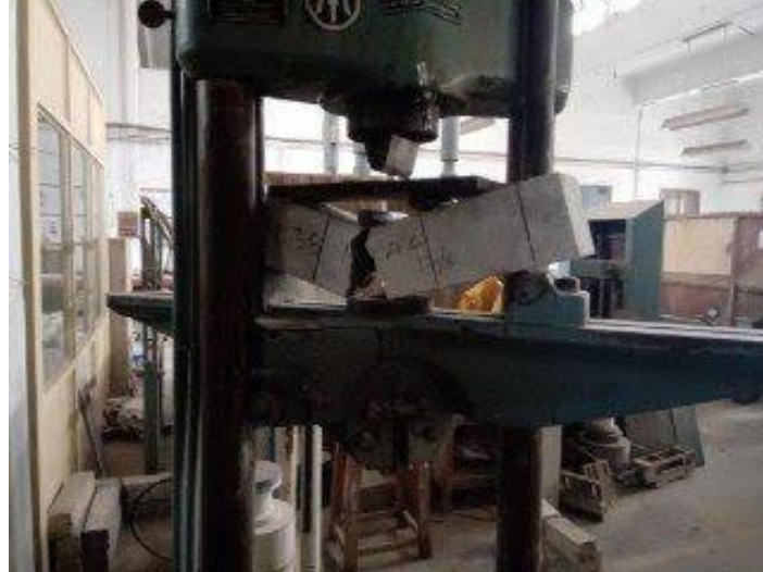
Figure 4.8 Flexural strength on prism
