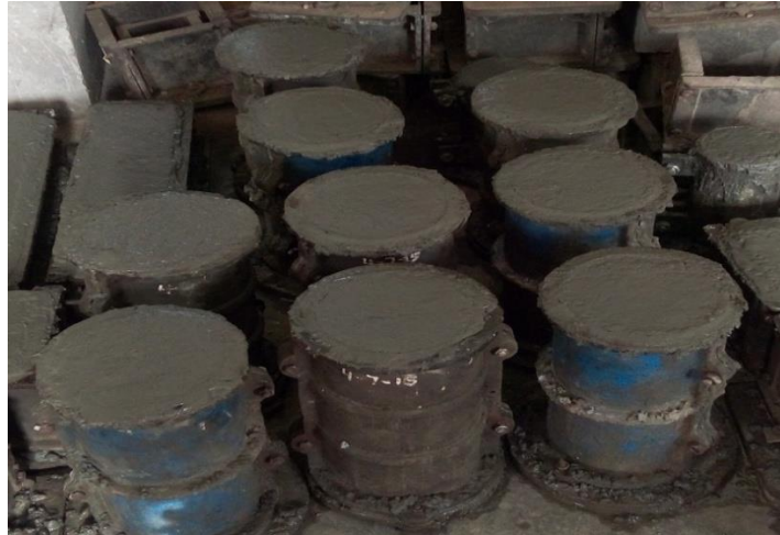
Figure 4.4 Casting of cylinders
