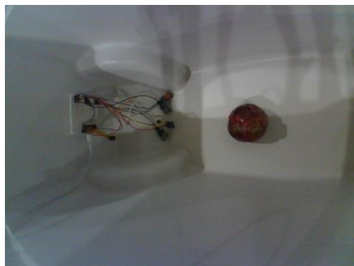
Figure 6: Rotten food tested in an ice box with a fisheye camera and gas sensors connected to an ESP32-S3 microcontroller.
