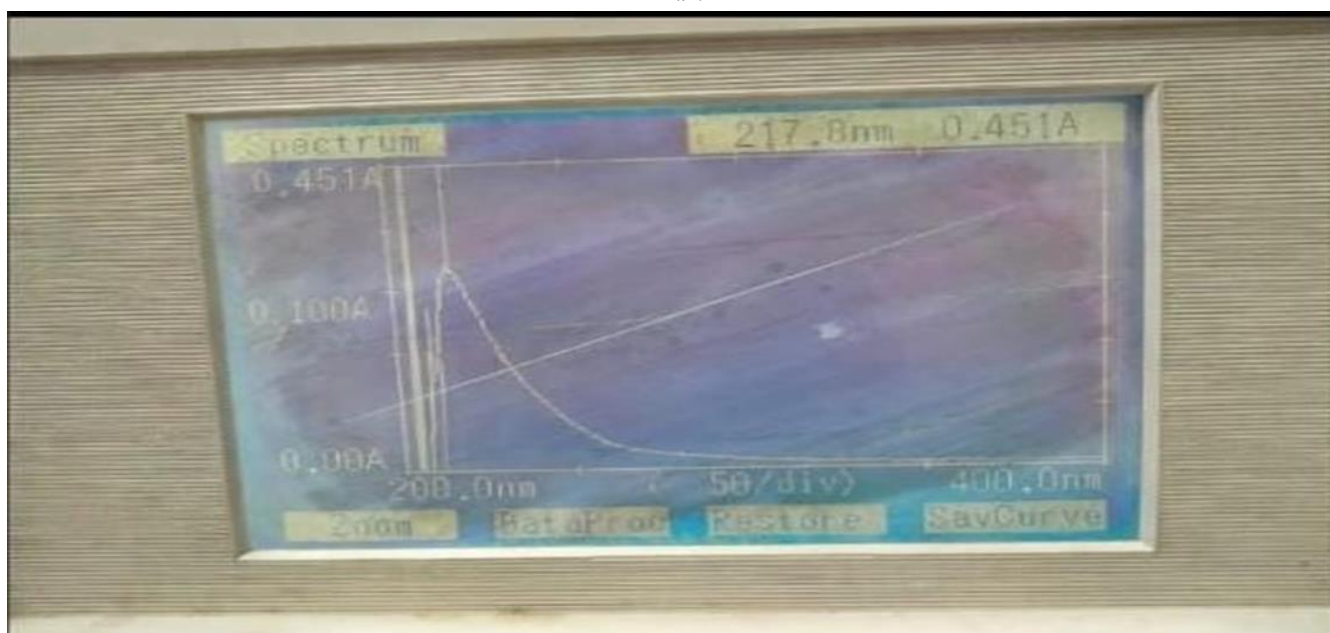
Figure 1: UV-Visible spectrum of Captopril ( \lambda_{\text{max of}}=217 nm).
