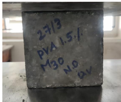
Figure 9.8 Salt immersed specimen after 28 days
