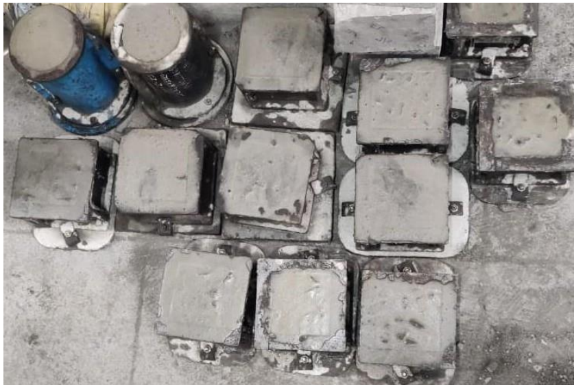
Figure 7.1 Casting of specimens
