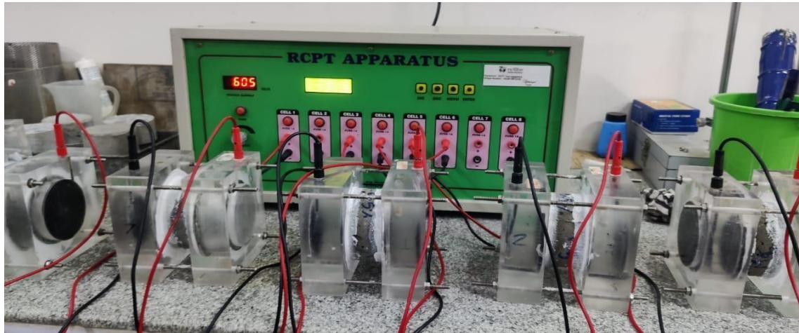
Figure 8.3 Test setup of Rapid Chloride Permeability Test
