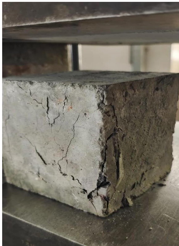
Figure 9.1 Compressive strength test
