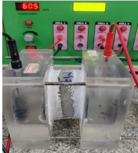
Figure 8.2 Specimen fixed in voltage cell
