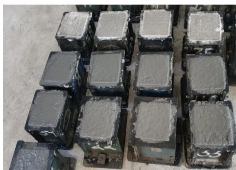
Fig 3.5.2 Filling of Concrete Mix in Cubes
