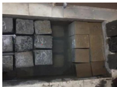
Fig 3.5.3 Curing of Concrete
