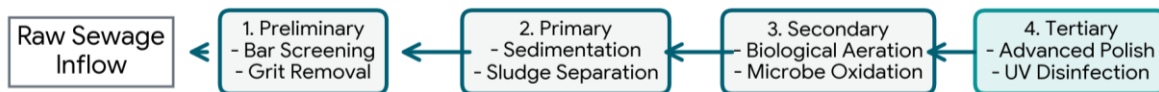
Figure 1: Simplified multi-stage processing architecture and unit operations flow inside a modern municipal sewage treatment plant.
